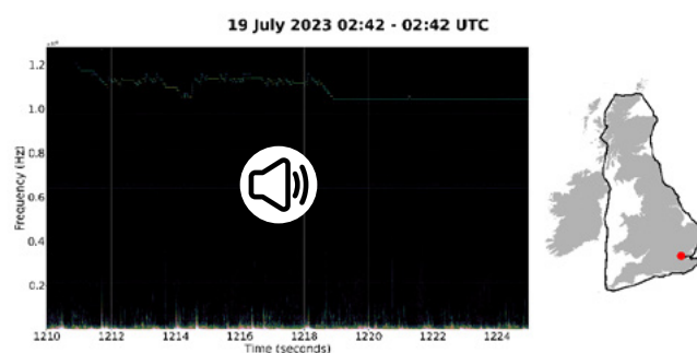
Visualisation and audio clips of the sound from an echosounder. The audio clip has been processed to make the high frequency sound audible and clearer, including a 50% reduction in speed.
